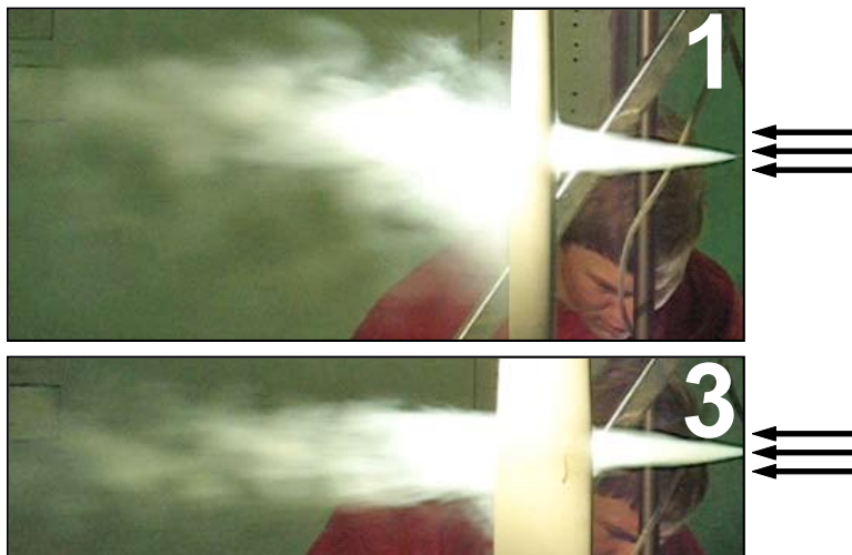
Figure 21: Side view images of the round (top, #1) and KVF (bottom, #3), illustrating the dramatic difference in wake size.
