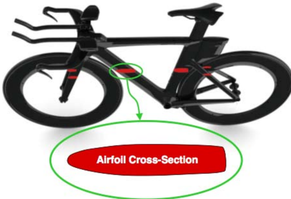
Figure 2: The Speed Concept with the 2D airfoil cross-sections of several tubes identified in red. Note that the airfoil is defined in the horizontal direction of the wind (waterline plane).
