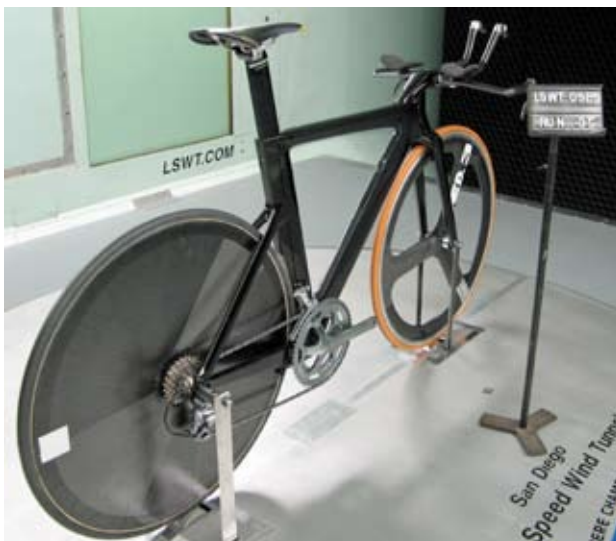
Figure 28: General setup from the June 2009 head-to-head wind tunnel tests. Notes: Team Speed Concept shown. Wheels would be spinning during the actual test. Bicycle yaw rotation is counterclockwise, such that the wind hits the drive side of the bicycle. San Diego Low Speed Wind Tunnel.
