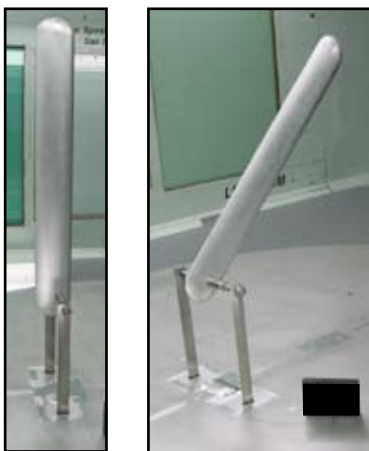
Figure 6: Top: Wind tunnel data showing the negative drag performance of two KVF designs at a vertical pitch angle. Bottom: Test images of an airfoil being tested at two different pitch angles. Notes: San Diego Low Speed Wind Tunnel. Tares removed (only the vertical struts and horizontal rod).
